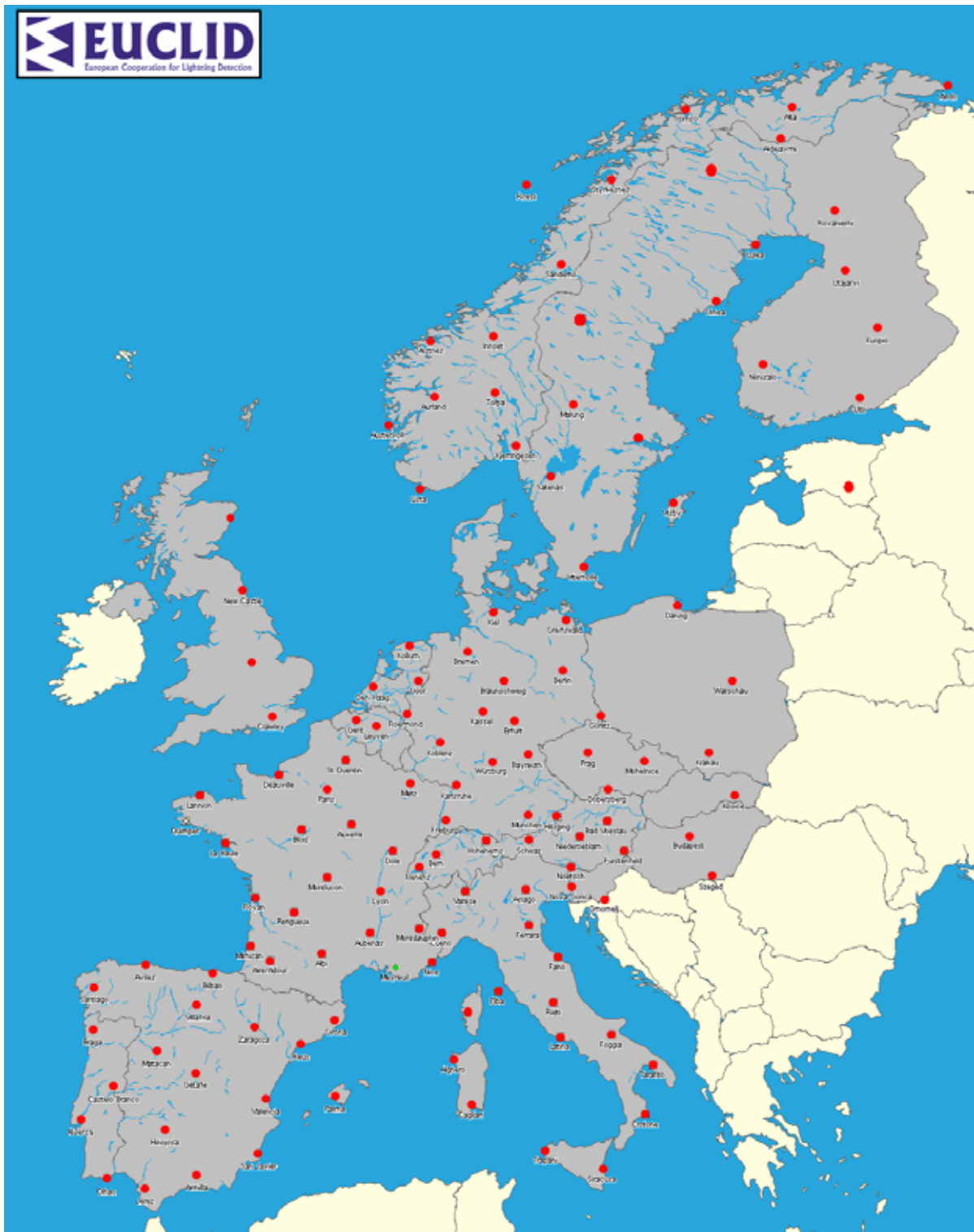
Fig.2. European Cloud to Ground Lightning detecting network EUCLID with marked location of detection sensors.
