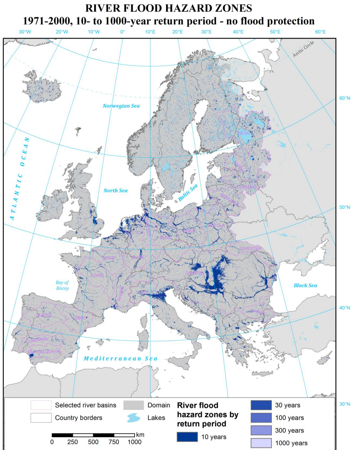
Fig. 7.5. River flood hazard zones by return period, historical scenario (1971-2000), no flood protection.
