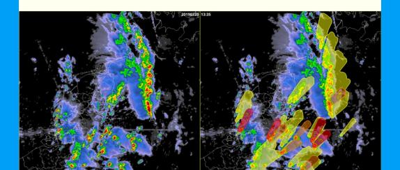
Warning polygons from the software I created at KNMI. Polygon colors are only based on column-maximum reflectivity however in this image.
