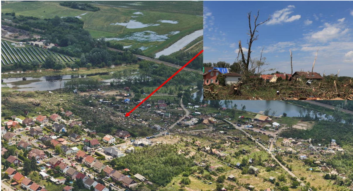
Aerial and ground photos showing a narrow swath of significant damage to the forest in southeastern Lužice. Note only light damage to the houses within 40 m of the swath. Photos: Lukáš Ronge and Tomáš Půčik.
