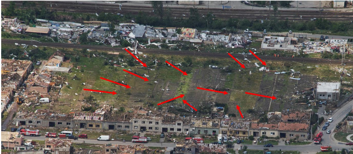
Aerial photo showing convergent debris patterns near the center of the tornado track in Mikulčice. Photo: Lukáš Ronge.
