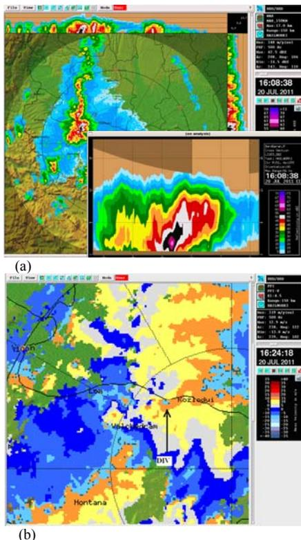
FIG. 6: Maximum development of storm A: (a) larger image – maximum reflectivity (dBz); smaller imbedded image –vertical cross-section of reflectivity (dBz) at 16:06 LT; (b) Doppler velocity (m/s) at 16:24 LT. The arrow points to the area of divergence.
