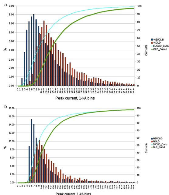
FIG. 8: The distributions of peak current for a) negative and b) positive strokes in Austria in July 2011.
