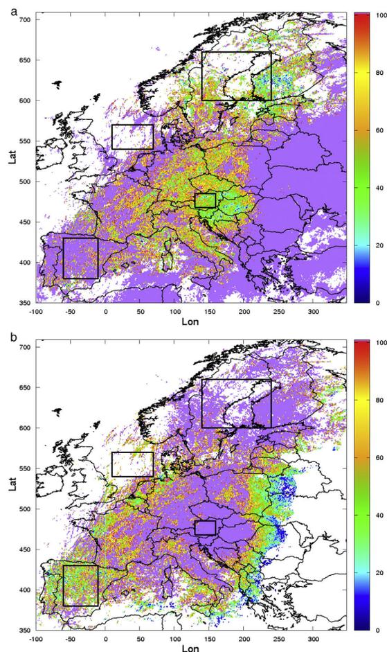
FIG. 3: Relative detection efficiency of a) GLD360 (the number of GLD360 strokes divided by the number of EUCLID CG strokes), and b) EUCLID (the number of EUCLID CG strokes divided by the number of GLD360 strokes), respectively. Study areas named Scandinavia, North Sea, Austria and Spain indicated with black squares from north to south respectively. Purple color indicates values larger than 100%.
