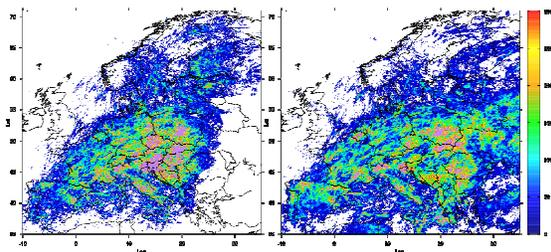
FIG. 1: Number of strokes in 0.1° longitude×0.1° latitude bins according to EUCLID (left) and GLD360 (right) during the study period. Purple color indicates values larger than 300 strokes.
