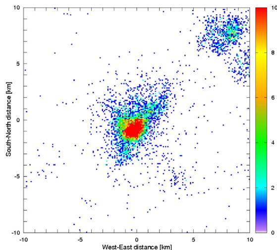
FIG. 5: Relative location accuracy of GLD360 compared to EUCLID in Austria in July 2011. The data set consists of a total of 9 418 temporally common strokes.
