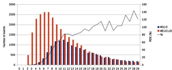
FIG. 4: Relative detection efficiency of GLD360 and for different peak currents in Austria in July 2011.
