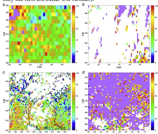
FIG. 2: Relative detection efficiency of GLD360 to EUCLID in a) Austria, b) North Sea, c) Scandinavia and d) Spain. Purple color indicates values larger than 100%.
