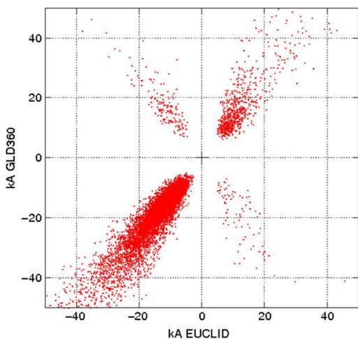
FIG. 7: Correlation between the measured peak currents of EUCLID and GLD360 for negative and positive temporally common strokes in Austria in July 2011.
