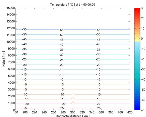
FIG. 2: Temperature profile [ $^{\circ}\text{C}$ ] at the initial time. The bulges represent the temperature perturbation.
