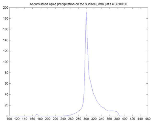
FIG. 9: Accumulated liquid precipitation at  $t = 06:00:00$  simulated time, using detailed microphysics.
