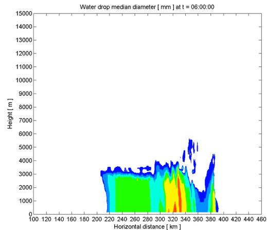
FIG. 5: Median volume diameter of water drops [ $\text{mm}$ ] at  $t = 06:00:00$  simulated time, using detailed microphysics. The dashed lines designate the temperature in  $^{\circ}\text{C}$ .
