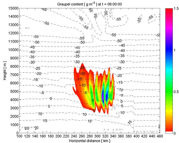
FIG. 7: Graupel particles content [ $\text{g m}^{-3}$ ] at  $t = 06:00:00$  simulated time, using detailed microphysics. The dashed lines designate the temperature in  $^{\circ}\text{C}$ .
