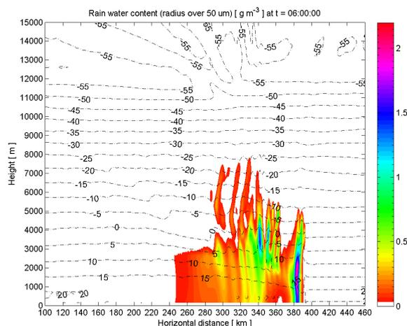
FIG. 3: Rain water (radius larger than  $50 \mu\text{m}$ ) content [ $\text{g m}^{-3}$ ] at  $t = 06:00:00$  simulated time, using detailed microphysics. The dashed lines designate the temperature in  $^{\circ}\text{C}$ .
