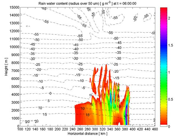
FIG. 3: Rain water (radius larger than  $50 \mu\text{m}$ ) content [ $\text{g m}^{-3}$ ] at  $t = 06:00:00$  simulated time, using detailed microphysics. The dashed lines designate the temperature in  $^{\circ}\text{C}$ .
