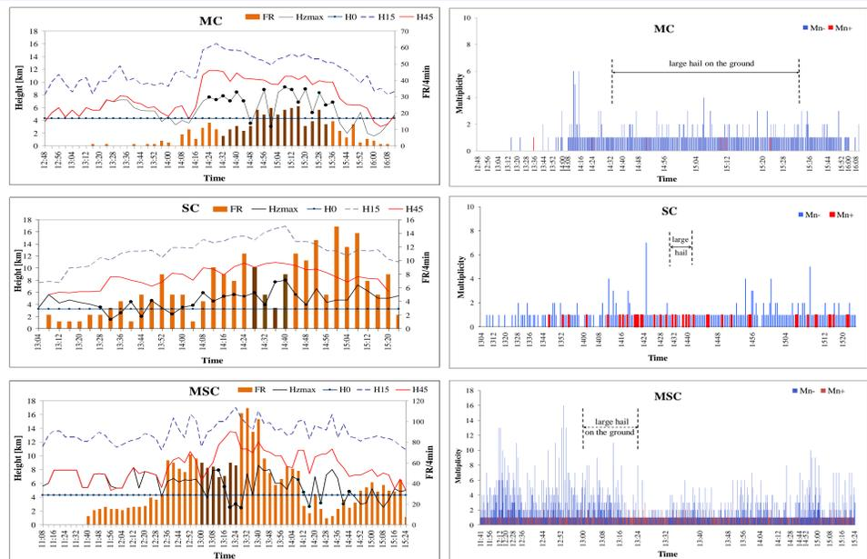
FIG. 1: Number of flashes per 4 minutes, FR, and radar information as a function of time. The FR during the period of intensive large hail on the ground is denoted by darker columns. The maximum radar reflectivity reached 60-65 dBZ is marked by dots on the curve of H<sub>zmax</sub>.
