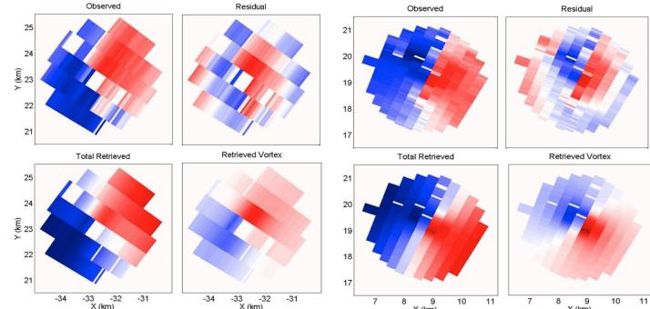
**Top Figure:** Wind retrieval of 30 May 2004 Geary, OK supercell using velocity data collected by two SMART radars. The retrieved vortex is embedded within a larger circulation (visible in the plots) that produced F-2 damage.
