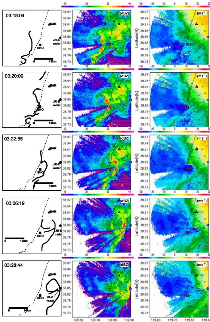
FIG.2 Color PPI scans of reflectivity (center) and Doppler velocity (right) from the JR-E radar located at the Amarume station at elevation angle of 3.0 at (a) 03:18:04 and (b) 03:26:19 LST. The bow and comma echo locations are shown in the left panel. The bold lines represent reflectivities greater than approximately 30 dBZ.
