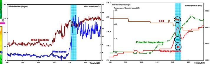
FIG. 4(a) Time series of surface wind speed and direction from the Shonai Airport. (b) Time series of surface pressure, temperature, and dewpoint depression (T-Td) from the Shonai Airport. The vertical hatches indicate the wind gust period.
