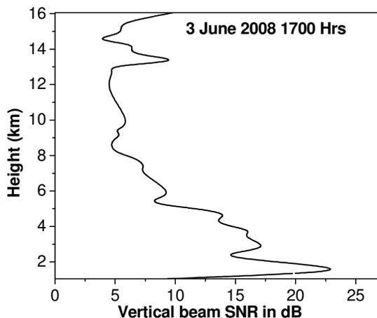
**FIG. 1: Vertical profile of hourly averaged vertical Beam SNR (in dB at 1700 Hrs on 3 June 2008) as derived from Pune wind profiler**
