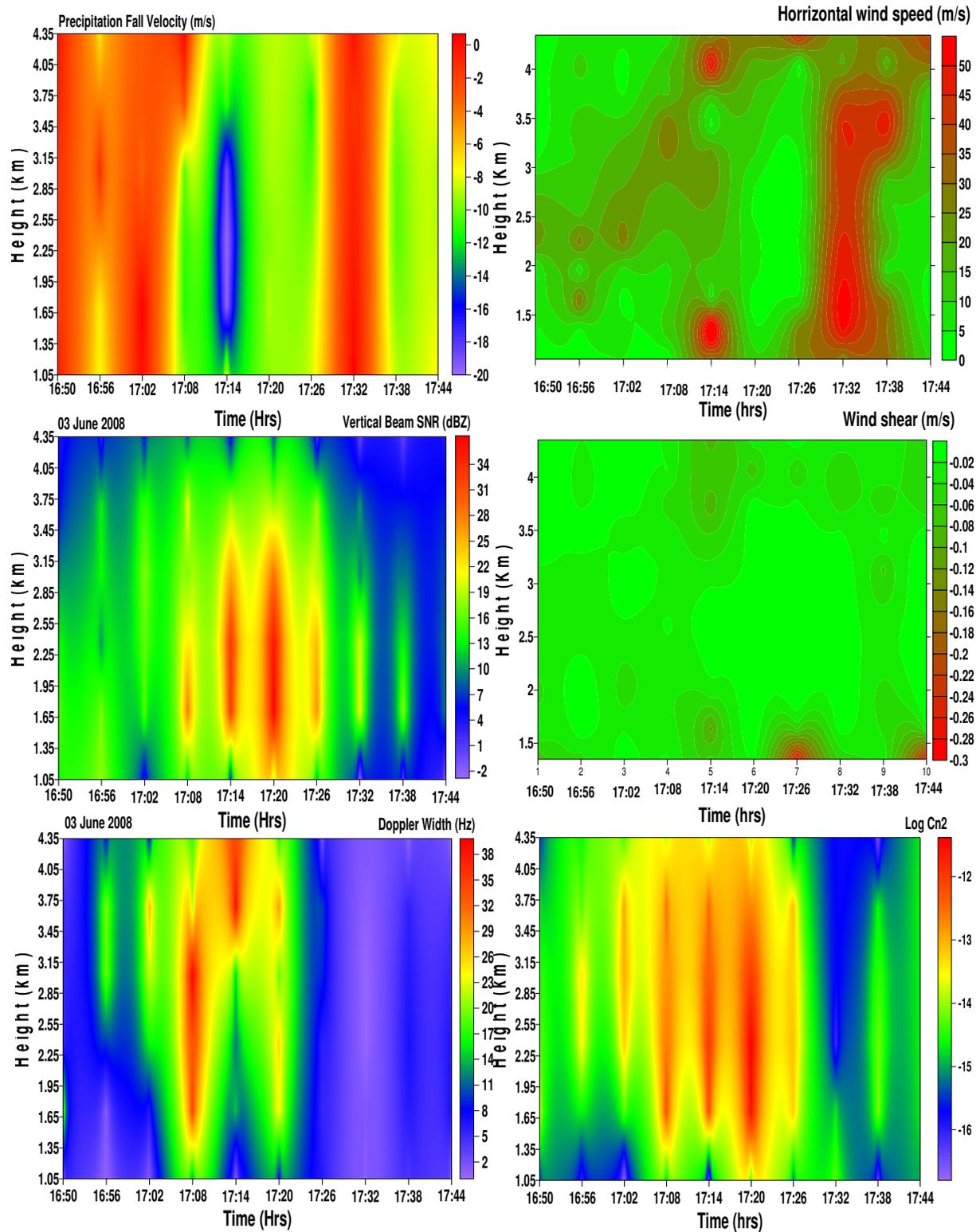
**FIG. 2:** Time height variations of wind profiler derived a: vertical motions, b: horizontal wind speed, c: vertical beam SNR, d: vertical shear of horizontal wind, e: spectral width and f: refractive index structure parameter (Figures in sequence from Top left to Bottom right – Figure 2a to Figure 2f).
