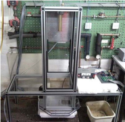
FIG. 4: Pneumatic hail gun with HARE below.
