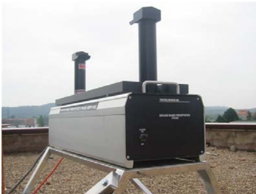
FIG. 1: Ground Based Precipitation Probe (PMI Model GBPP-100) installed at the University of León.
