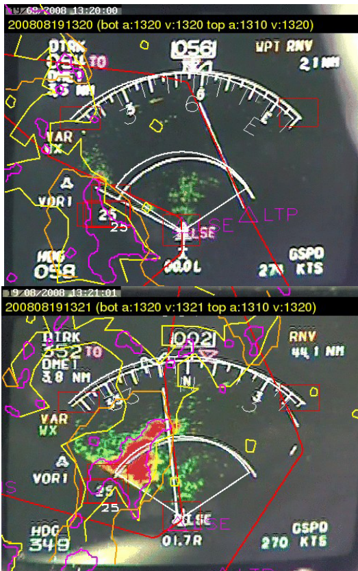
FIG. 3: On board display of radar images (colored shading) and CB WIMS objects (colored contours) during a sharp turn. Cb top objects are indicated in orange, Cb bottom objects with severity "moderate" in yellow and with severity "severe" in magenta. The flight path of the aircraft is marked by a red line with the aircraft's position indicated by a white aircraft symbol. LSE is a waypoint near Lyon. Top image at 13h20'00" on August 19th, bottom image 61 seconds later. Objects are diagnosed using data from 13h20.
