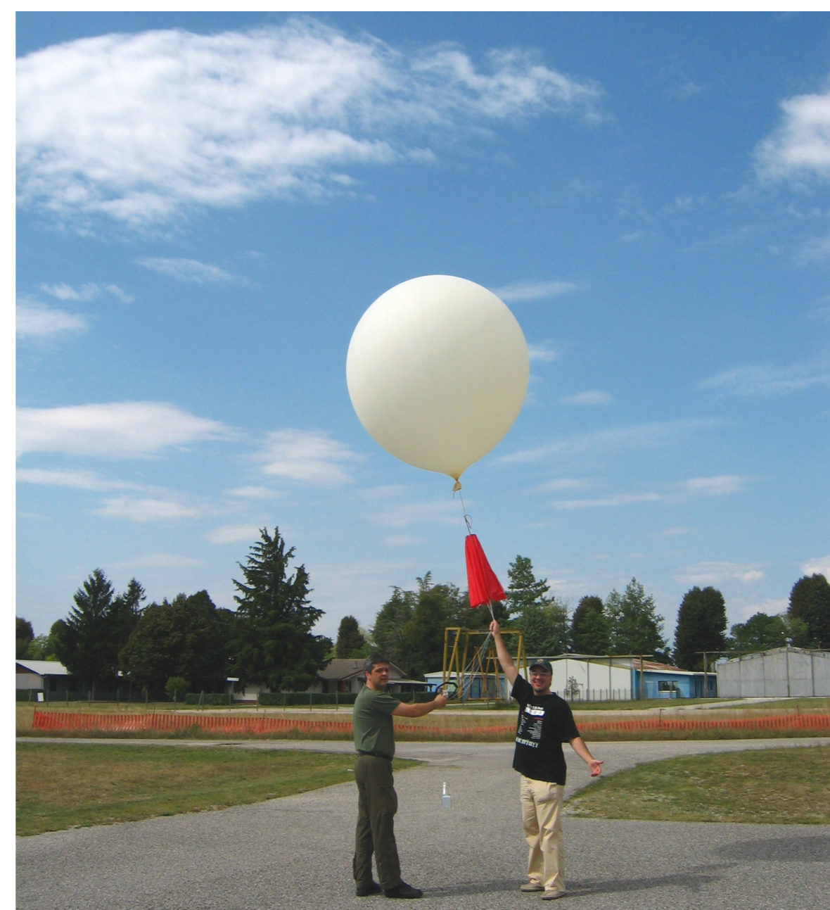
20090910 12UTC radiosounding launch from the Udine station of A.M. using a Vaisala RS-92 sonde (courtesy of M. Mariano).
