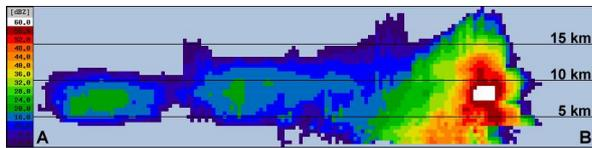
FIG. 2b: Radar reflectivity vertical cross-section A-B of the storm in Fig. 2a. The cross section ranges from ground up to 20 km, lines indicate 5, 10 and 15 km CAPPI levels. Note that the high echo top is located outside the CWC.
